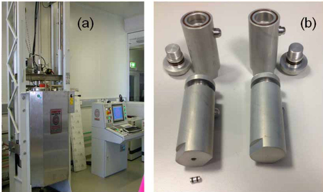
Figure 1: (a) Stansted High Pressure unit utilised in this study; (b) “Pressure on” (left) and “Pressure off” (right) devices manufactured from high tensile strength aircraft aluminium for the investigation of the high pressure effect on thermal spore inactivation.
